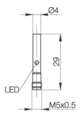
**Inductive Sensors** BES G04EC-NSC15B-S26G D4 x 29 normally-open **Sn=1,5mm** shielded
